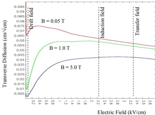
Fig. 2. Transverse diffusion coefficient for Ar CH<sub>4</sub> (95:5) as a function of electric field for three magnetic fields as calculated by the MAGBOLTZ [5] program. Significantly larger diffusion is possible in the induction and transfer gaps, as compared to the drift volume, for high magnetic field operation.
