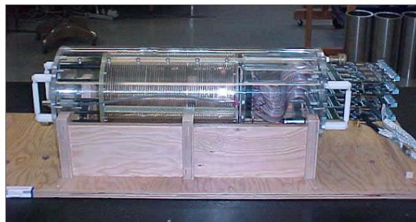
Fig. 4. Photograph of TPC2, located at the University of Victoria. Located on the right endcap are front end cards produced for the STAR TPC.
