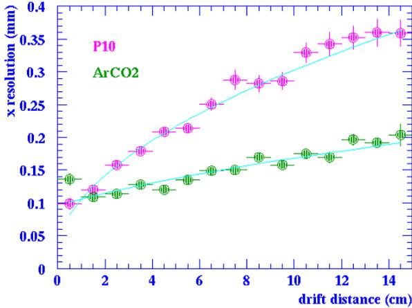
Fig. 6. Resolution in the horizontal component as a function of drift distance for TPC1. The lowest drift distance bin contains only a few events.
