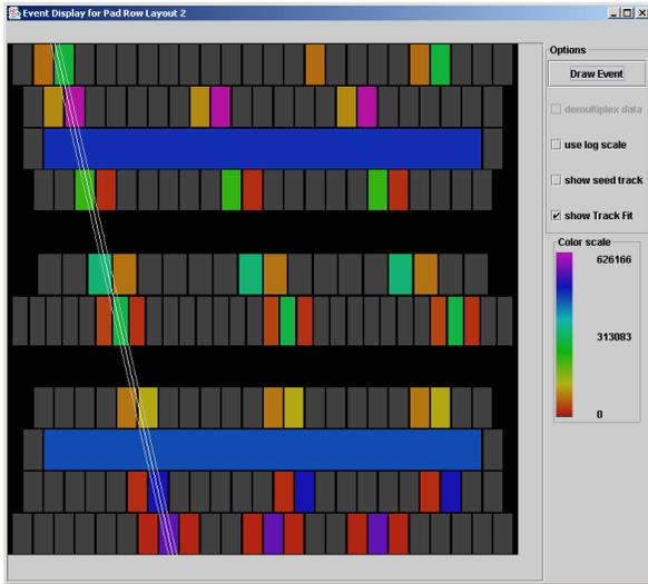
Fig. 5. Event display from a cosmic ray event recorded by TPC1. The color of the pads represents the size of the signal recorded by the corresponding electronics channel (see scale on right). Three fold multiplexing was used.
