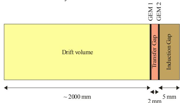
Fig. 1. Concept of a large scale TPC, such as that envisaged for a future linear collider experiment. The electric field in the drift volume is parallel to the magnetic field, resulting in low transverse diffusion for the drifting electrons. In the transfer and induction gaps, the transverse diffusion is significantly larger, which will help spread the charge over a larger region as they are collected by the pads at the endplate.
