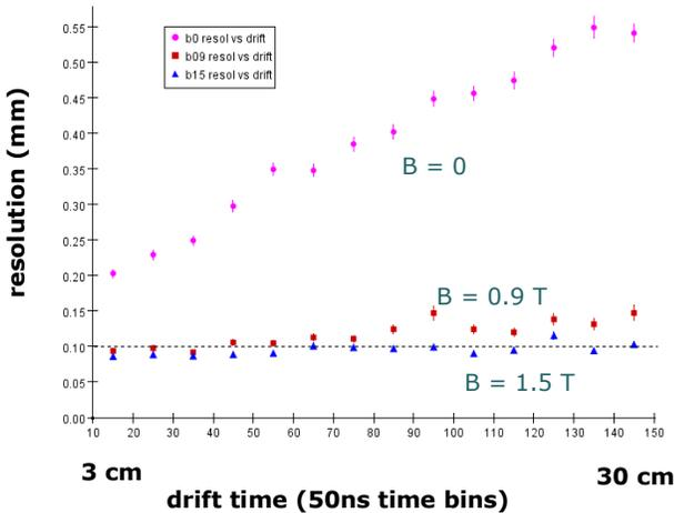
Fig. 9. Resolution (mm) is shown as a function of drift time (50 ns time bins) for TPC2 in Ar CH<sub>4</sub> (95:5). The horizontal axis corresponds to drift distances between 3 and 30 cm. The results shown here are to be considered preliminary.
