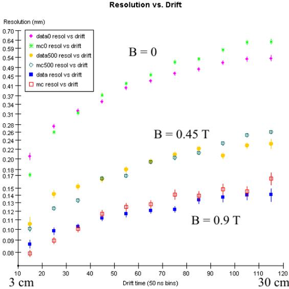
Fig. 9. Resolution (mm) is shown as a function of drift time (50 ns time bins) for TPC2 in Ar CH<sub>4</sub> (90:10). The horizontal axis corresponds to drift distances between 3 and 30 cm. The solid points correspond to real data, the open points are from simulated data. The results shown here are to be considered preliminary.
