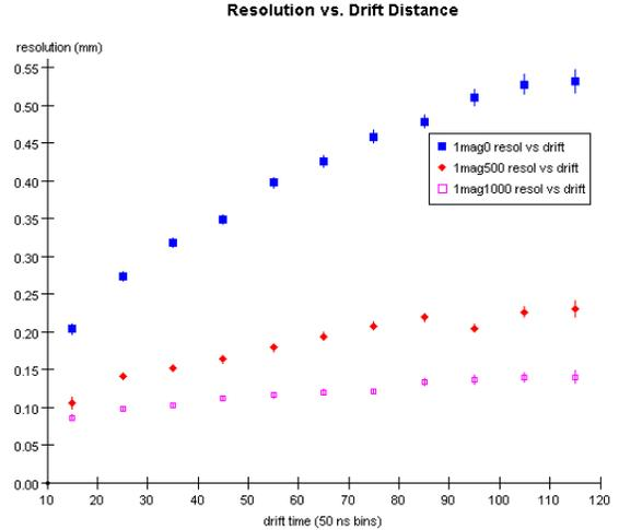
Fig. 8. Resolution (mm) is shown as a function of drift time (50 ns time bins) for TPC2 in Ar CH<sub>4</sub> (90:10). The horizontal axis corresponds to drift distances between 3 and 30 cm. The upper (blue) points are at zero field, the middle (red) points are at 0.45 T, and the lower (magenta) points are at 0.9 T. These data are from a preliminary analysis.
