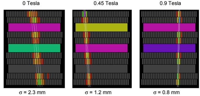
Fig. 7. Event displays from cosmic ray events recorded by TPC2 at TRIUMF. The color of the pads represents the size of the signal recorded by the corresponding electronics channel. Each track drifted about 25 cm. Below the displays are shown the standard deviation of charge distribution about the track as determined by the track fit.
