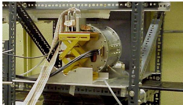
Fig. 3. Photograph of TPC1, located at Carleton University. The scintillator paddles that form the cosmic ray trigger are visible.
